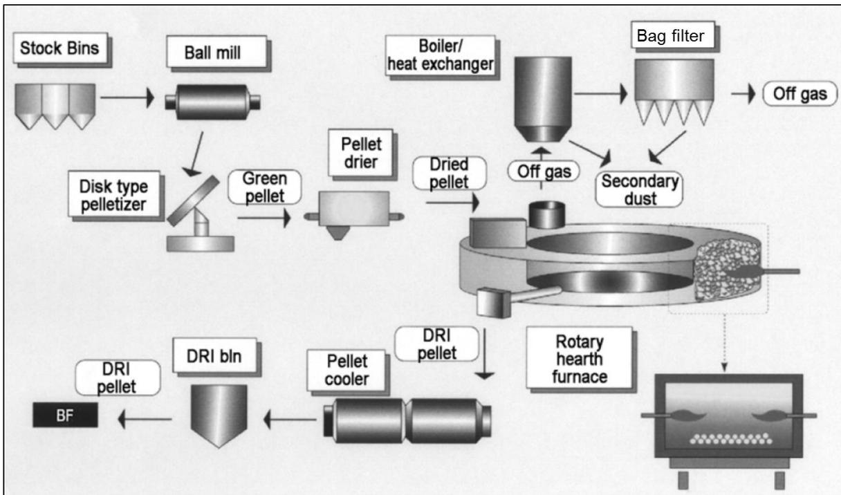
The Rotary hearth furnace technology is a proven technology developed from the end of the 20<sup>th</sup> century.
